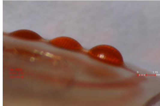
Fig5.Side view of the adjustable microlens on the hemi-sphere substrate.
