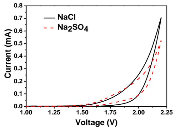
Fig. 4 IV curves of electrolysis by using Na<sub>2</sub>SO<sub>4</sub> and NaCl as the electrolytes. (working electrode: ITO, counter electrode: BiVO<sub>4</sub> film, reference electrode: calomel)
