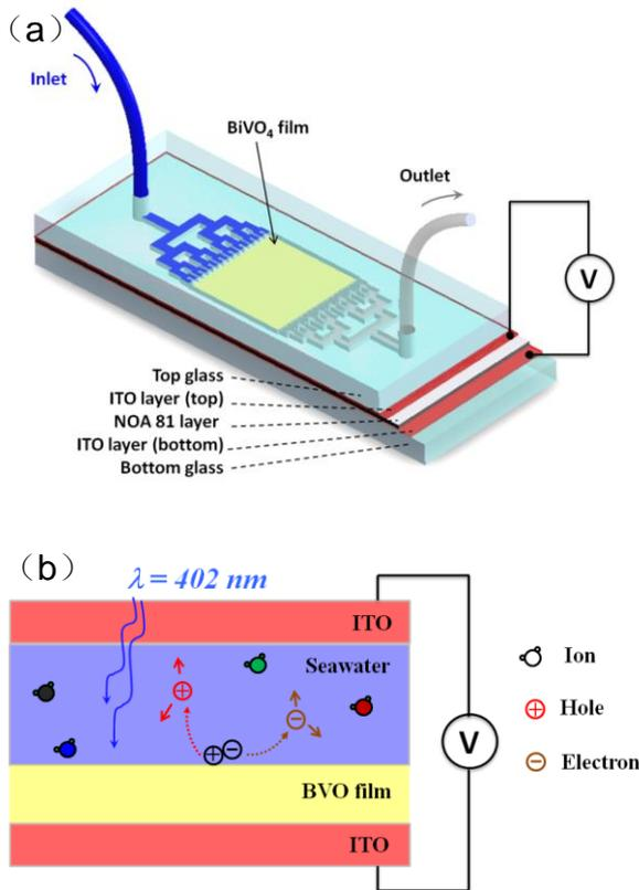
Fig.1 (a) Schematic diagram of the microfluidic planar reactor and structures of the catalyst film and the tree-shaped microchannels for inlet and outlet. (b) the cross section of the PEC microreactor.
