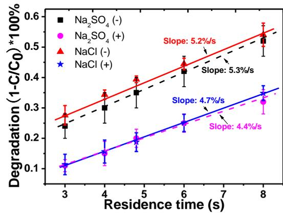
Fig. 3 Influence of the flow rate on the degradation efficiency of microreactor under ±1.8 V external bias by using NaCl (solid lines) and Na<sub>2</sub>SO<sub>4</sub> (dash lines) as the electrolyte.
