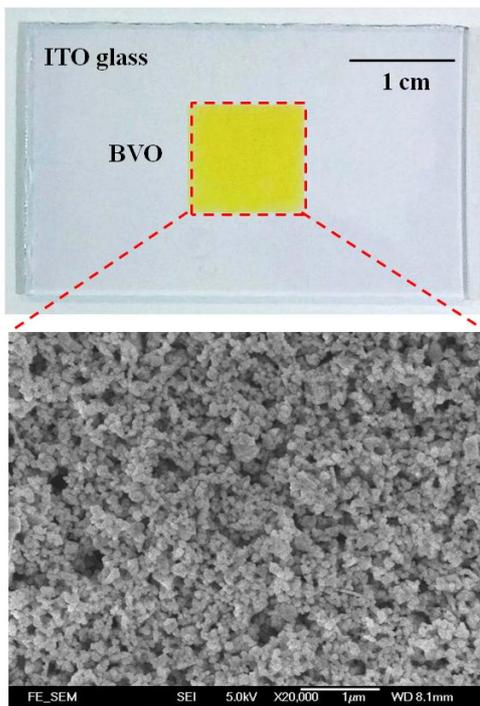
Fig. 2 The upper panel: the BiVO<sub>4</sub> film on the ITO glass slide. The lower panel: SEM photo of the BiVO<sub>4</sub> film, which shows the nanoporous structure.
