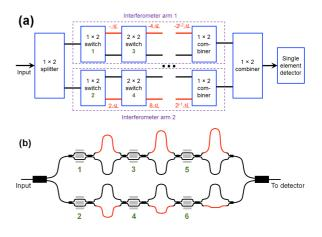
Fig. 2 (a) Block diagram of the dFTIR spectrometer design; (b) schematic layout of a 64-channel dFTIR spectrometer: the waveguide segments of varying lengths different from the standard length are shown in red (not drawn to scale). The green numbers label the  $1 \times 2$  or  $2 \times 2$  switches.
