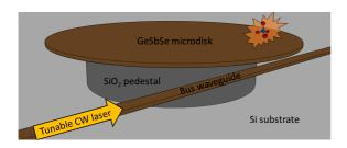
Fig.1 Schematic of a suspended microdisk cavity structure for sensing a target gas molecule in the surrounding air. Brown denotes a 30  $\mu$ m radius Ge<sub>23</sub>Sb<sub>7</sub>Se<sub>70</sub> microdisk coupled to a bus waveguide, all suspended 10  $\mu$ m above a Si substrate by SiO<sub>2</sub> supports.
