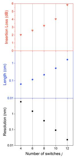
*Fig. 3 Projected spectral resolution, interferometer arm length and insertion loss of the dFTIR spectrometer.*
