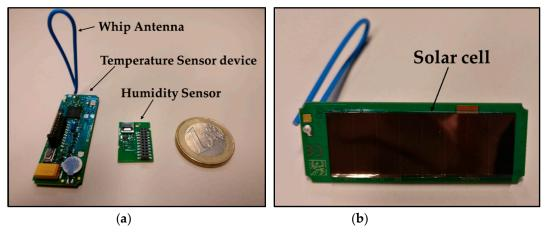
**Figure 2.** (a) EnOcean's STM 330 module and the includable humidity sensor; (b) Detail of the STM 330 module's solar cell.
