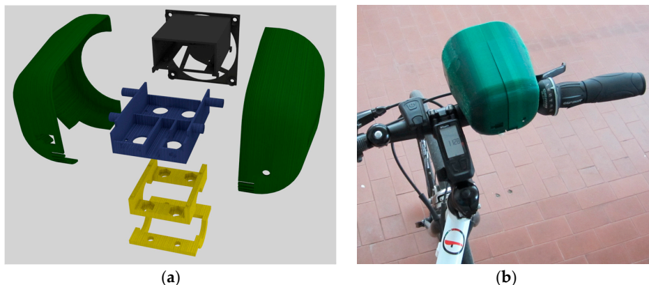
Figure 1. Monitoring system: (a) assembly scheme rendering; (b) as installed.
