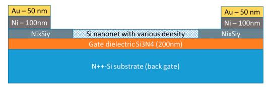
Figure 1. Cross-Section of Si Nanonet FET
