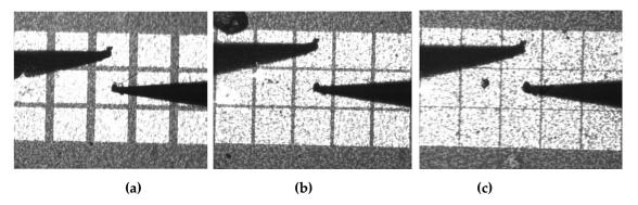
Figure 2. Pictures of (a) 30μm, (b) 15μm, and (c) 5μm channel gap Si nanonet FETs
