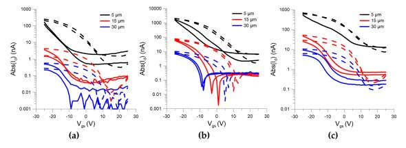
**Figure 3.** The  $I_d$ - $V_{gs}$  curves for **(a)** low density, **(b)** medium density and **(c)** high density Si nanonet FETs under and gate voltage up (solid lines) and down (dashed lines) sweeps and a drain voltage of  $V_{ds} = -4 \ V$ .
