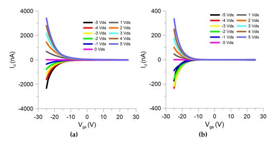
**Figure 6.** The up-sweep  $I_d$ - $V_{gs}$  curves for medium density  $5\mu m$  nanonet channel FETs measured in **(a)** March and **(b)** September 2017
