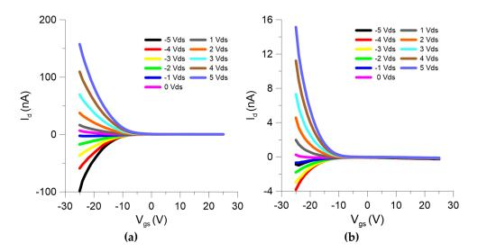
**Figure 5.** The up-sweep  $I_d$ - $V_{gs}$  curves for medium density 15 $\mu$ m nanonet channel FETs measured in (a) March and (b) September 2017
