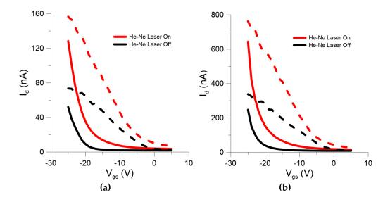
**Figure 4.** The Id-Vgs curves of the high density Si nanonet FETs when irradiation with He-Ne Laser was set on and off under gate voltage up (solid lines) and down (dashed lines) sweeps and a drain voltage of (a)  $V_{ds}$  = 1V and (b)  $V_{ds}$  = 5V
