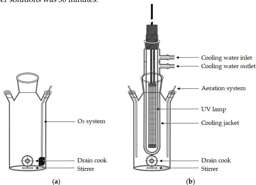
**Figure 1.** Reactor for the (a)  $\text{H}_2\text{O}_2$ ,  $\text{O}_3$  and (b) UV, UV/ $\text{TiO}_2$  [10] process
