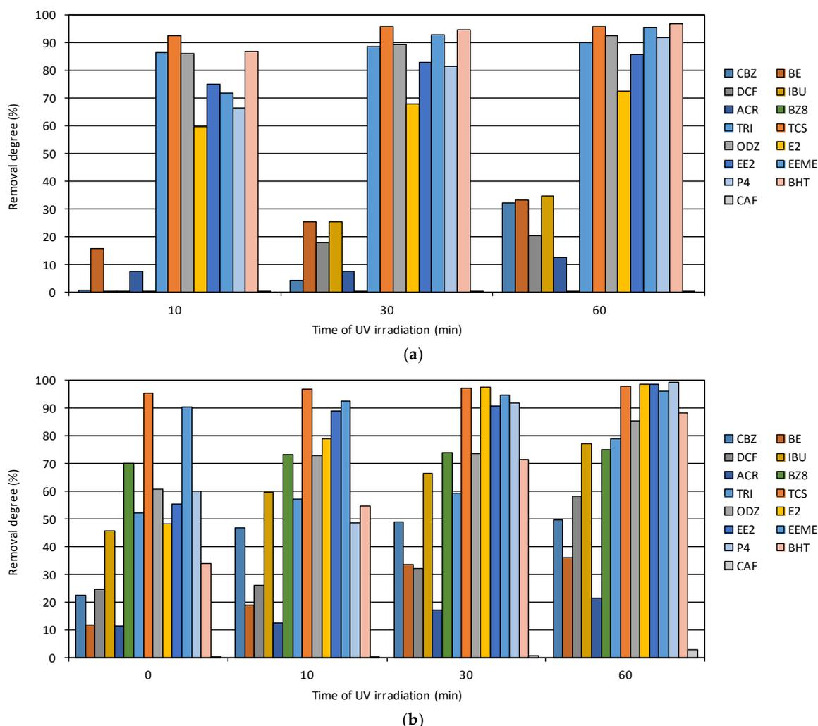
Figure 3. Degradation of micropollutants in the (a) UV and (b) UV/TiO<sub>2</sub> process
