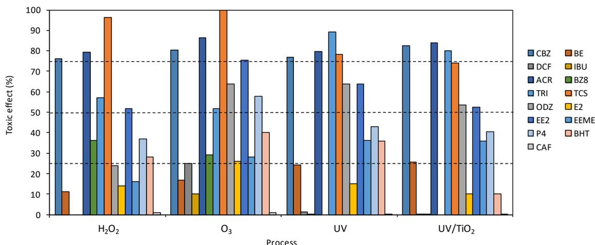
Figure 5. Change in toxicity o micropollutant water solution after selected oxidation processes
