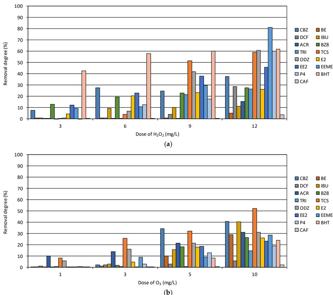
**Figure 2.** Degradation of micropollutants in the (a) H<sub>2</sub>O<sub>2</sub> and (b) O<sub>3</sub> process
