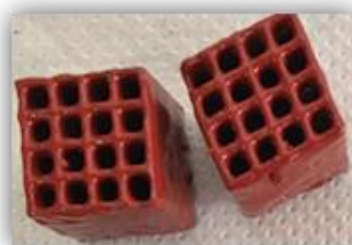
Figure 5. Ceramic monolithic filter (200 cpsi) coated with a silicone based coating containing tethered Ectocarpus (<math><0.6\text{ wt.}\%</math>).
