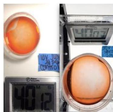
**Fig. 4:** From left to right: Side by side comparisons during a 10 volt trial where the left is the assay and the right is the control. The picture on the left shows a deceleration of the oscillating process of the BZ reaction.
