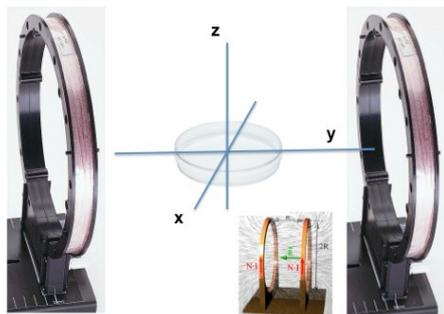
**Fig. 1:** Experimental setup to study the influence of the magnetic field on the BZ reaction.
