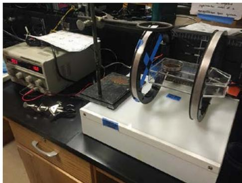
**Fig. 1:** DC power supply which is connected to the Helmholtz coil. A petri dish is placed on top of a suspended flask to ensure that the solution is directly in the most uniform area.
