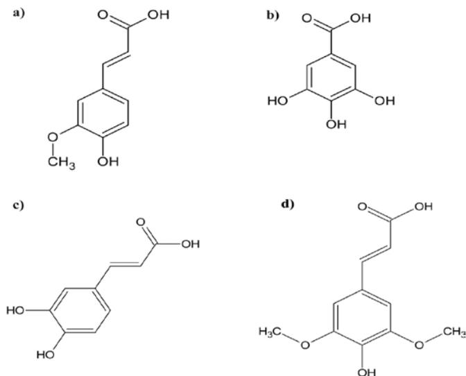
**Figure 1.** Chemical structure of phenolic compounds a) ferulic acid b) gallic acid c) caffeic acid and d) sinapic acid
