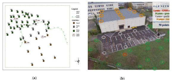
Figure 1. (a) The spatial distribution of the 50 GCPs and the study area limit in the local coordinatesystem, (b) UAS image with the location of the 50 GCPs.
