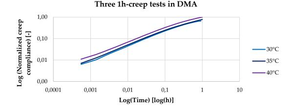
**Figure 5:** Creep curve of PA6, performed from 23 °C until 45 °C in 5 °C steps created from DMA test with a load according to 0.1 % of the tensile strain at a strain rate of 10<sup>-5</sup>s<sup>-1</sup>
