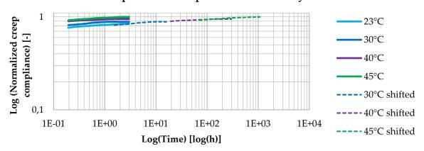
Four 3h-creep tests enable prediction of 100 days
