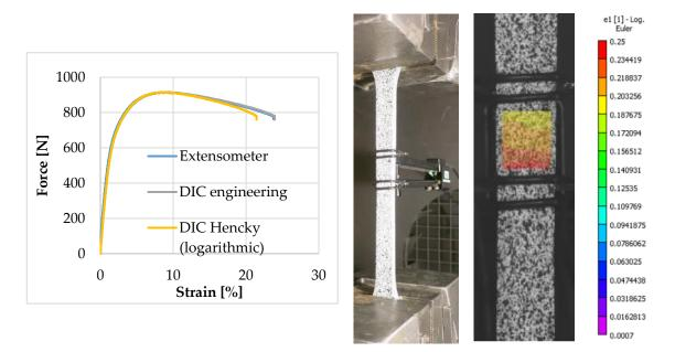
Figure 2: Comparison of DIC and extensometer measurement, good result until Fmax
