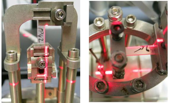
Figure 7: Aligned laser lines for straighter sample mounting in tensile clamp and single cantilever
