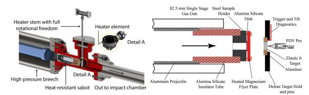
**Figure 1 (a).** Schematic of the custom designed heater system with axial and rotational degrees of freedom at the breech-end of the gas gun
