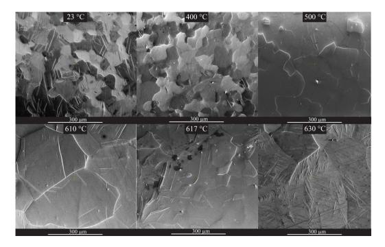
**Figure 4.** SEM images of 99.9% commercial pure magnesium showing the central region on the cross-section of shock compressed samples recovered from normal plate impact experiments.
