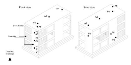
**Figure 1**. Isometric view of building. Location of pressure gauges, accelerometers, the displacement gauge and the explosive charge [6].
