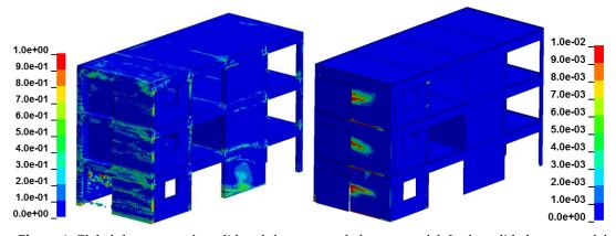
**Figure 4.** Global damage on the solid and the structural element model. In the solid element model red elements indicate failed elements due to either ductile or brittle damage. In the structural element model red areas indicate locations where reinforcement bars have higher plastic strains than 1%.
