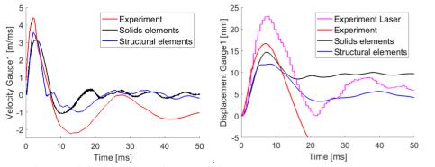
**Figure 5.** Velocity and displacement in horizontal direction at gauge A1 from the experiment and the numerical simulations with solid and structural elements for the first 50 ms.
