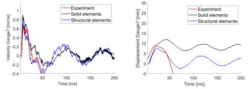
**Figure 3.** Velocity and displacement in horizontal direction at gauge A7 from the experiment and the numerical simulations with solid and structural elements.
