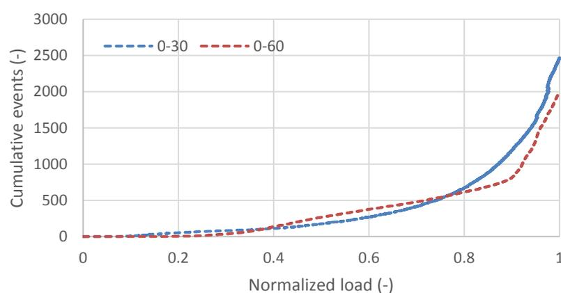
**Figure 2.** Total AE events recorded for the two laminates during the static tests.
