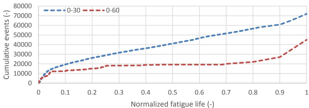
**Figure 4.** Total AE events recorded for the two laminates during the fatigue life for a 70% test.
