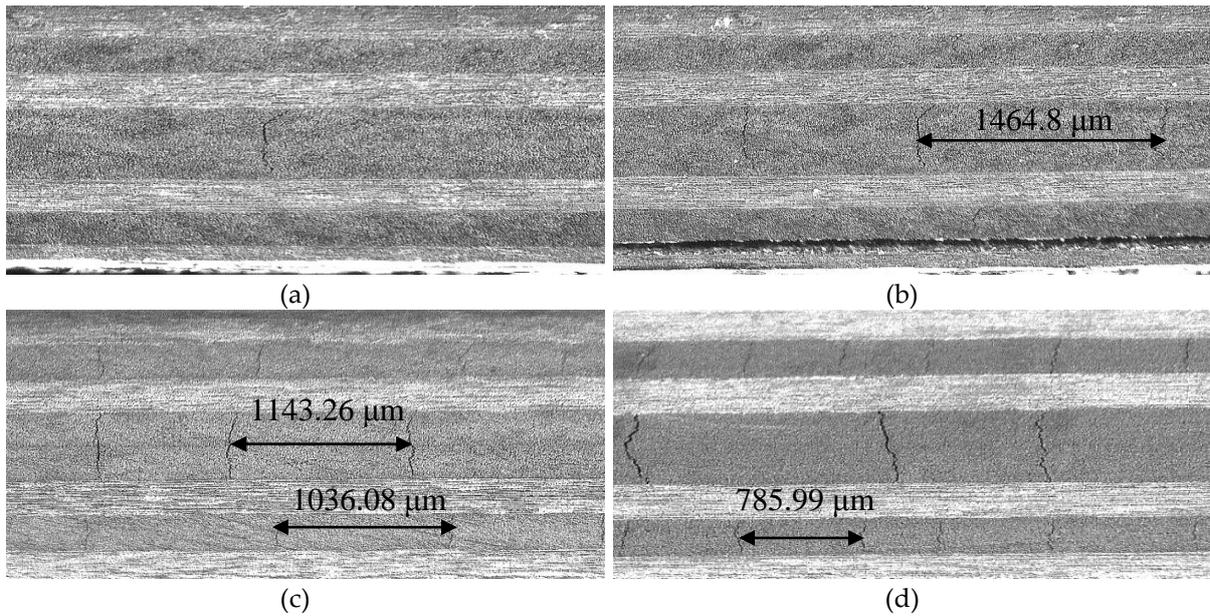
**Figure 3.** Fatigue damage state at 70% maximum load for  $[0^\circ/30^\circ]_{2s}$  laminates after (a) 10 cycles and (b) 200 cycles and for  $[0^\circ/60^\circ]_{2s}$  laminates after (c) 10 cycles and (d) 200 cycles.
