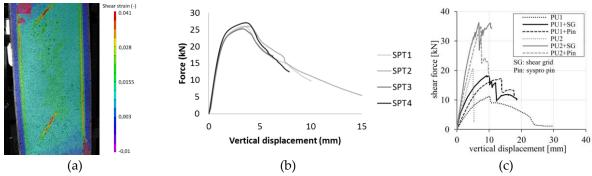
**Figure 6.** (a) shear failure at a load of 40 kN, (b) force-displacement curve of the double-lap shear test with a thinner core of 20 mm , (c) double-lap shear test performed by Shams et el. [1]
