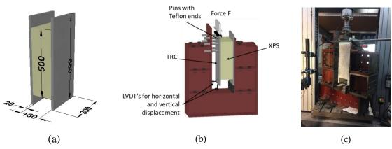
**Figure 1**. (a) specimen geometry and dimensions in mm, (b) schematic presentation of the double-lap shear test, (c) picture of double-lab shear test
