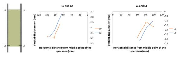
Figure 5. initiation of debonding (line L0) at a load of 22kN
