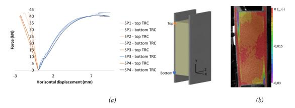
**Figure 4.** (a) horizontal displacement (x-direction) of the top and bottom of the loaded TRC face, (b) compression at the interface
