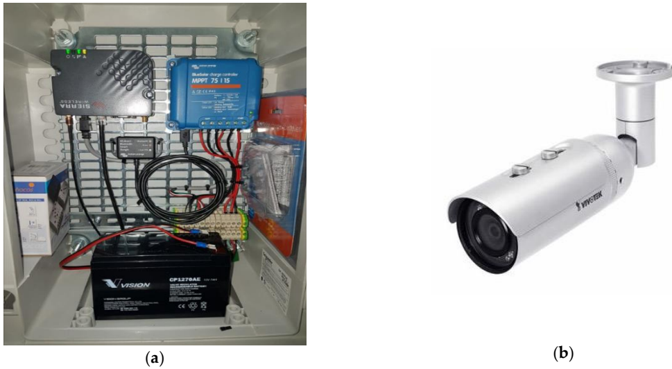
Figure 4. (a) Sierra Wireless RV50 router, Victron Energy BlueSolar charge controller MPPT 75 115, and Battery 12-24v 75 v 29a trickle charger cabinet, (b) the IB8369 IP-camera from Vivotek Inc.
