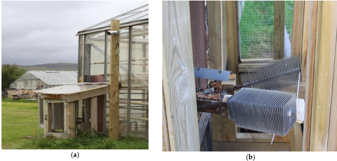
Figure 2. At the Agricultural University of Iceland near Hveragerdi, (a) two co-joined exterior sheds were attached to a greenhouse to enclose and protect (b) the three thermoelectric generators (two shown).
