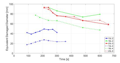
**Figure 4.** Equivalent damaged diameter area time evolution for the Temperature Difference Method.
