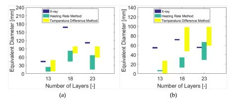
**Figure 3.** Comparison of the quantitative values of equivalent damaged diameter for the three techniques presented. (a) specimens impacted with the 9 mm projectile and (b) with the .357 projectile.
