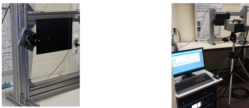
Figure 2 The experimental setup: The CFRP plate connected to the electro-magnetic shaker & Scanning Laser Doppler vibrometer (SLDV)
