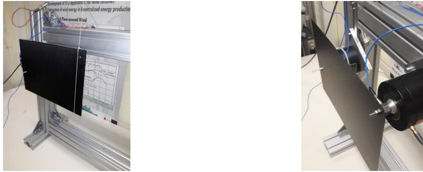
Figure 3 Two different boundary condition scenarios: the plate is fixed on one side and free suspended on the other side (i.e. a free-attached boundary condition) (left); the plate is fixed to two shakers (right)
