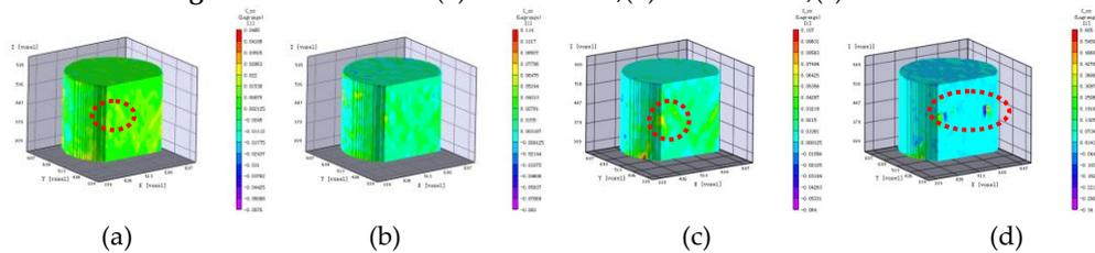
Fig. 12  $\epsilon_{xx}$  strain field of section b. (a)  $\sigma = 6.62$  MPa; (b)  $\sigma = 7.23$  MPa; (c)  $\sigma = 7.38$  MPa
