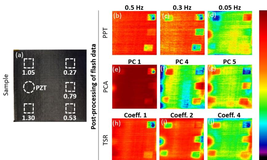
**Figure 5:** (a) CFRP sample with inserts (with defect depths indicated (in mm)), PPT images at: (b-d) 0.5, 0.3 Hz and 0.05 Hz, PCA images: (e-g) 1<sup>st</sup>, 4<sup>th</sup> and 5<sup>th</sup> PC, TSR polynomial coefficients for an interpolation order of 5: (h-j) 1<sup>st</sup>, 2<sup>nd</sup> and 4<sup>th</sup> coefficient.
