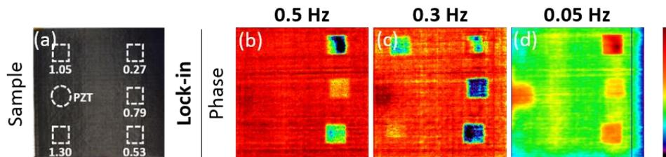
**Figure 4:** (a) CFRP sample with inserts (with defect depths indicated (in mm)), phase images from lock-in at: (b-d) 0.5, 0.3 and 0.05 Hz.
