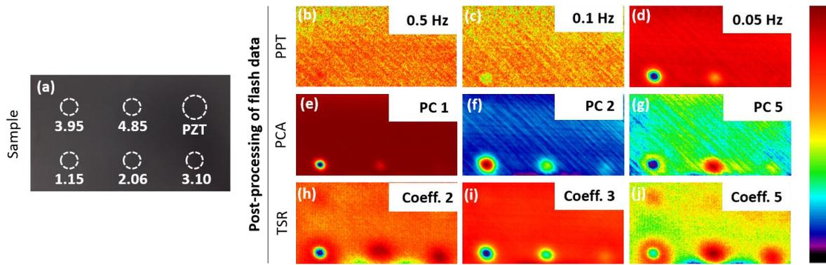
**Figure 3:** (a) CFRP sample with FBH's (with defect depths indicated (in mm)), PPT images at: (b-d) 0.5, 0.1 and 0.05 Hz, PCA images: (e-g) 1<sup>st</sup>, 2<sup>nd</sup> and 5<sup>th</sup> PC, TSR polynomial coefficients for an interpolation order of 5: (h-j) 2<sup>nd</sup>, 3<sup>rd</sup> and 5<sup>th</sup> coefficient.
