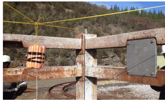
Figure 2. (a) Sketch of the aluminium plate showing its dimensions and the position of the three pressure gauges; (b) instrumented plate with three pressure gauges ready for the test
