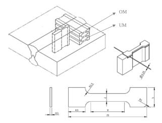
Figure 3: Extraction and dimensions of micro tensile specimens
