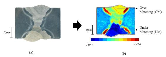
**Figure 1:** (a) weld section extracted from S690 test plate and (b) hardness (HV5) contour plot obtained from sample shown in (a) with approximately 1000 indents
