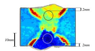
**Figure 2:** The AWMTT specimens were extracted at a 2mm distance from the plate surfaces in the OM and UM regions. They were extracted such that the entire cross section lies within the weld without intersecting the HAZ or the interface between OM and UM weld metal.
