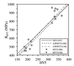
Figure 4: Hardness values (HV5) against tensile strength  $(R_{\rm m})$  from different transfer functions and experimental data
