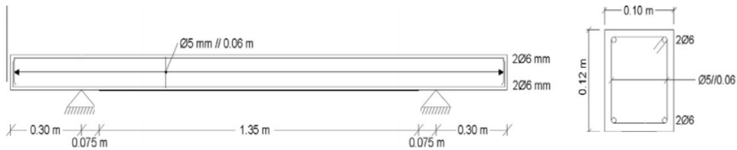
Figure 5. Geometry of the tested beam 2 "test specimen 2" [2]
