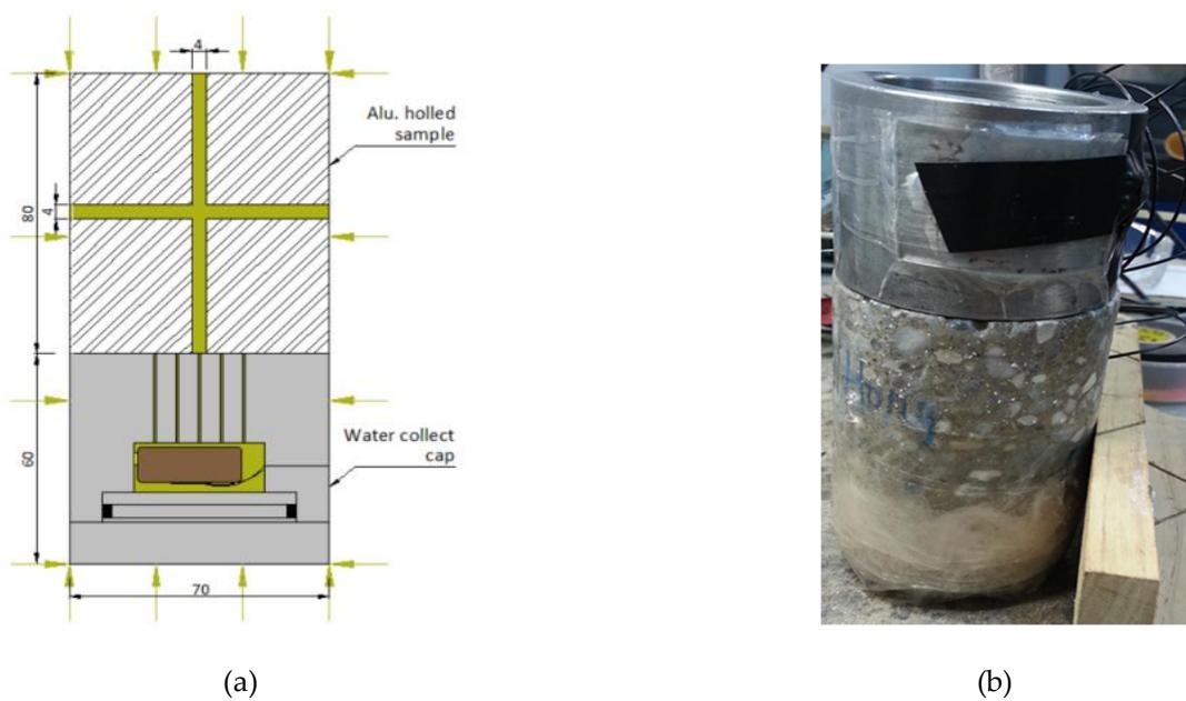
Figure 3: Experimental set up: (a) calibration test concept (b) pore pressure test preparation
