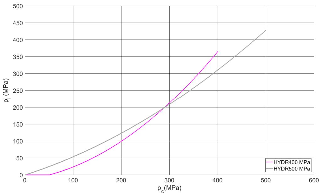
Figure 4: Pore pressure tests result: pore pressure  $\varnothing$  vs. confining pressure  $\varnothing$
