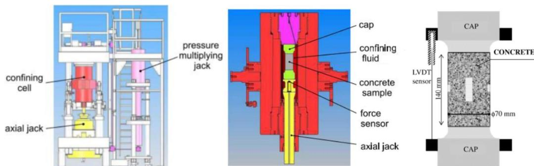
Figure 1: GIGA press (a) general view (b) section of the confining cell (c) sample instrumentation
