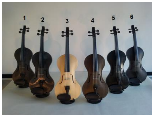
Figure 3: Six prototype violins with soundboards made from different materials
