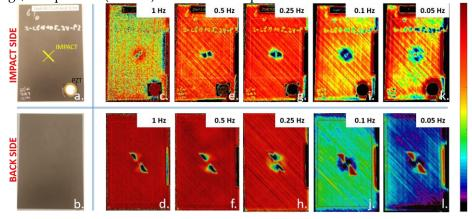
Figure 7: IRT in reflection of impact side (top row) and backside (bottom row) of CFRP<sub>BVID</sub>: (a-b) photograph; phase images at (c-d) 1 Hz, (e-f) 0.5 Hz, (g-h) 0.25 Hz, (i-j) 0.1 Hz and (k-l) 0.05 Hz.
