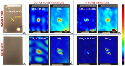
Figure 6: Results of impact side (top row) and backside (bottom row) of CFRPBVID: (a-b) photograph of sample, (c-d) out-of-plane LDRz and frequency band data FBDz over 2-100 kHz and (e-f) in-plane LDRxx and frequency band data FBDxx over 2-100 kHz.
