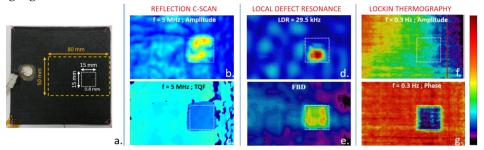
Figure 4: Results for CFRP<sub>INSERT</sub>: (a) photograph of inspected area. Ultrasonic C-scan at 5 MHz: (b) reflected amplitude and (c) TOF. Vibrational testing: (d) LDR at 29.5 kHz and (e) frequency band data FBD over 5-100 kHz. Lock-in thermography at 0.3 Hz: (f) amplitude and (g) phase image.
