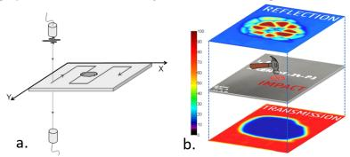
Figure 1: (a) Principle of C-scan and (b) ultrasonic C-scan in reflection (top) and transmission (bottom) for an impacted [45/0/-45/90]<sub>35</sub> CFRP (middle) with impact energy 18.5 J. The color scale indicates the amplitude level.
