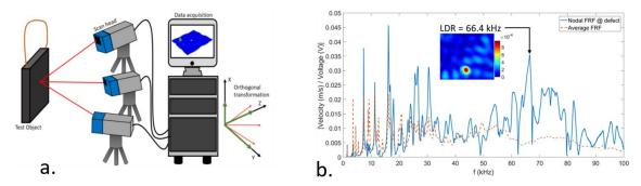
Figure 2: (a) Principle of 3D scanning laser Doppler vibrometry and (b) FRF of a [45/0/-45/90]<sub>3S</sub> CFRP sample with a flat bottom hole (diameter of 10 mm).
