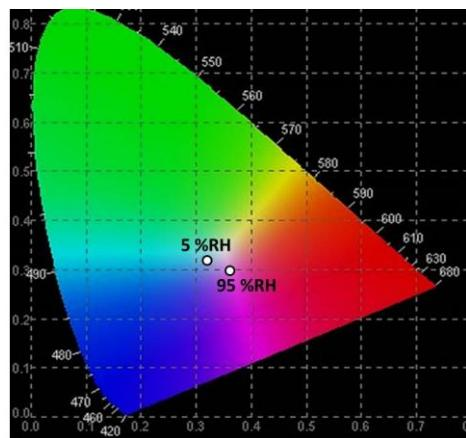
**Figure 5.** CIE color coordinates for polymer films with thickness of 290 nm deposited on 5-layers Bragg stack comprising  $\text{SiO}_2$  and  $\text{Nb}_2\text{O}_5$  films at denoted values of relative humidity.
