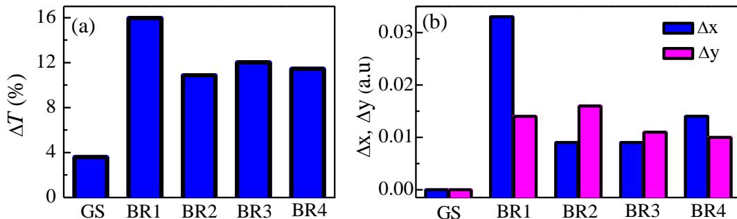
**Figure 4.** Humidity induced changes in transmittance (a) and CIE color coordinates  $x$  and  $y$  (b) for single polymer film with thickness of 290 nm deposited on bare glass substrate (GS) and on Bragg reflectors (BR) (BR1-5 layers, BR2-7 layers -  $Nb_2O_5$  and  $SiO_2$ ; BR3-5 layers, BR4-7 layers – dense and mesoporous  $Nb_2O_5$ ).
