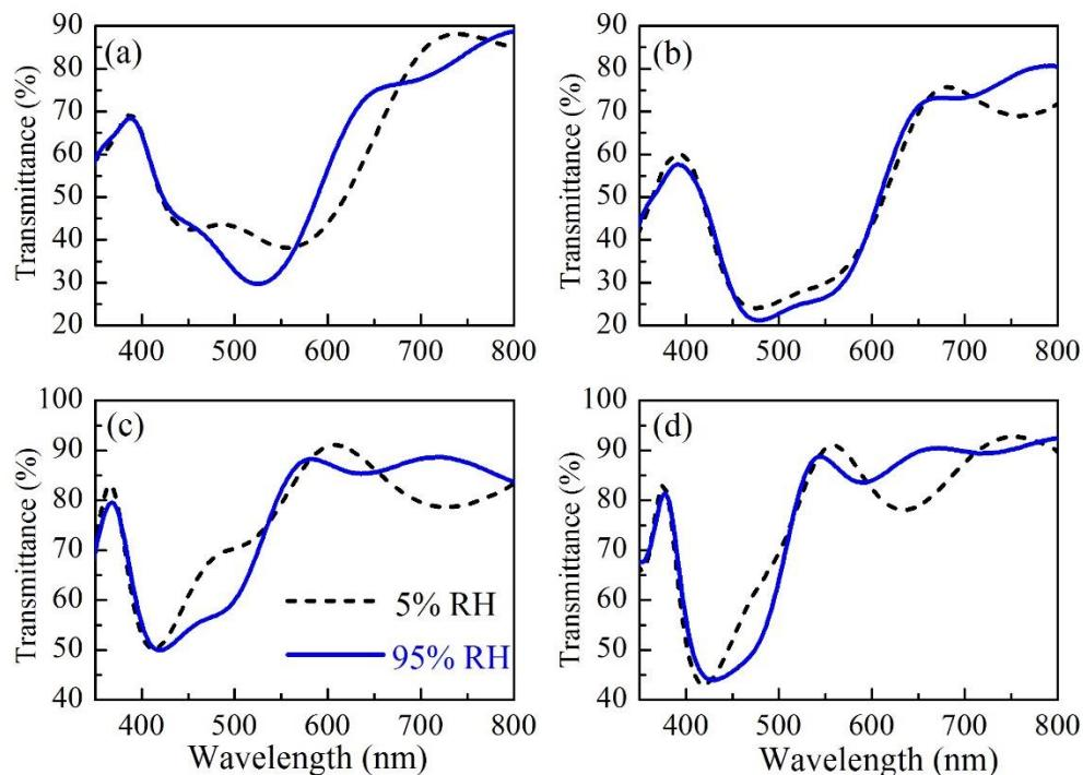
**Figure 3.** Transmittance spectra at low (5%) and high (95%) relative humidity of branched polymer film with thickness of 290 nm deposited on top of Bragg reflectors consisting of 5 (a, c) and 7 (b, d) alternating layers of  $\text{Nb}_2\text{O}_5$  and  $\text{SiO}_2$  (a, b) and dense and mesoporous  $\text{Nb}_2\text{O}_5$  (c, d)
