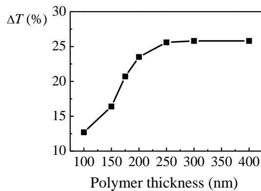
**Figure 1.** Calculated humidity induced change of transmittance  $\Delta T$  ( $=T_{95\%RH}-T_{5\%RH}$ ) of 5-layers Bragg reflector covered with polymer film with different thicknesses.
