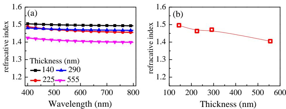
**Figure 2.** (a) Dispersion curves of refractive index of polymer films with denoted thicknesses; (b) thickness dependence of refractive index (the values are taken at wavelength of 600 nm).
