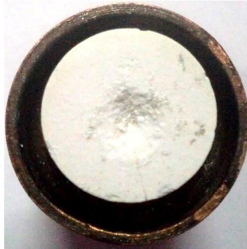
□  $\text{ZrO}_2$  pellet fixed at top of the anode is brought into ionized state by hot and dense argon plasma producing material ions.
