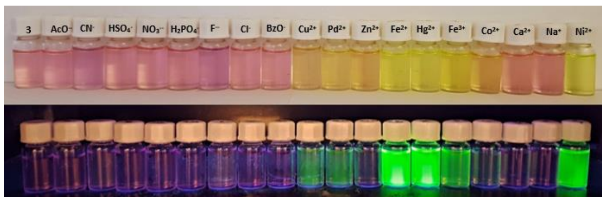
Figure 4. Evaluation of BODIPY derivative 3 as colorimetric (top) and fluorimetric (bottom) chemosensor for several ions in acetonitrile solutions.
