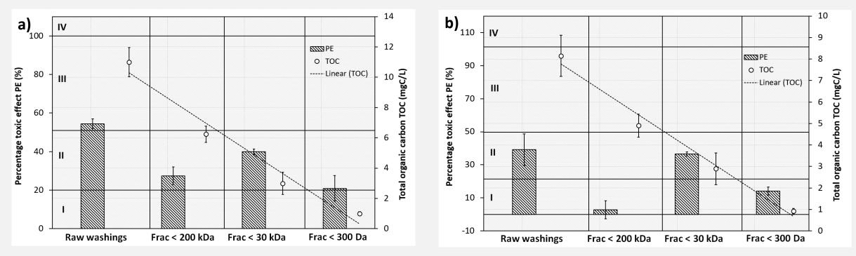
Fig. 6. Values of TOC and PE in raw washings and separated fractions, samples were taken from: (a) swimming pool—sampling 2.
