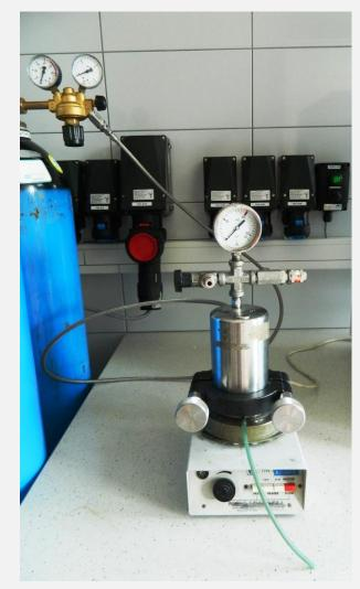
Fig. 2. The steel filter cell for membrane filtration
