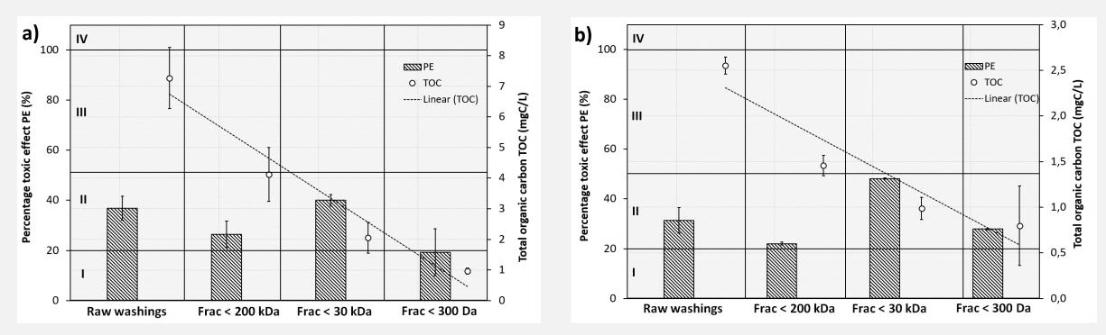
Fig. 7. Values of TOC and PE in raw washings and separated fractions, samples taken from: (a) hot tub—sampling 1; (b) hot tub—sampling 2.
