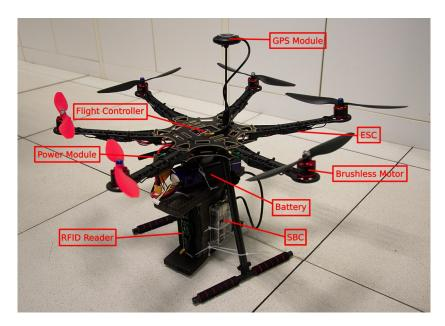
Figure 2. UAV used by the inventory and traceability system.
