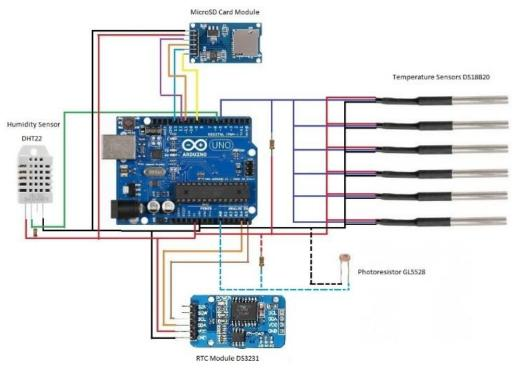
Figure 1. Electrical diagram of the thermodynamic monitoring system.
