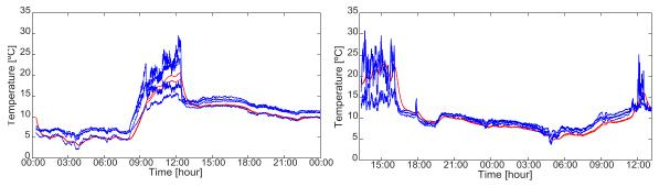
**Figure 6.** Temperatures obtained in situ (blue line) and by simulating with COMSOL (red line). Results of the wood box (left). Results of the polystyrene box (right).
