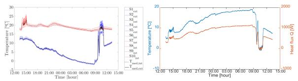
**Figure 7**. East wall results. At left, temperatures obtained inside (blue) and outside (red). At right, heat flow (orange) and temperature (light blue).
