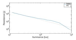
**Figure 5.** Difference between the value of each sensor and the reference thermometer (left). Relation between resistance (right, blue line) and illuminance on a photoresistor and a linear fit (right, dotted line).
