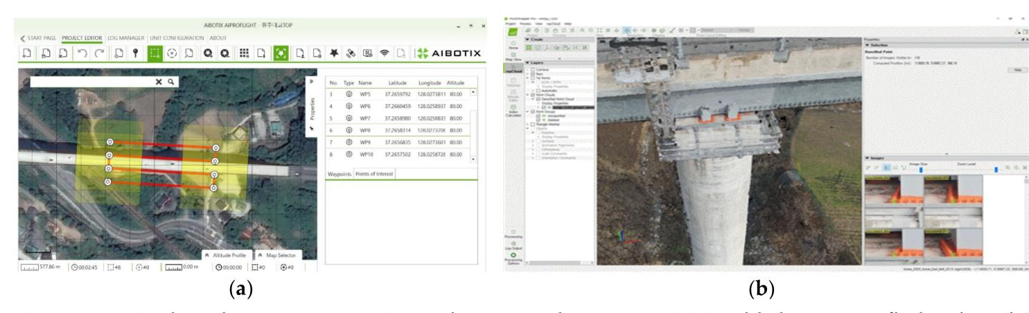
Figure 3. UAV based monitoring in Wonjudaegyo Bridge, Korea: (a) Establishing UAV flight plan; (b) Sample image taken by UAV.
