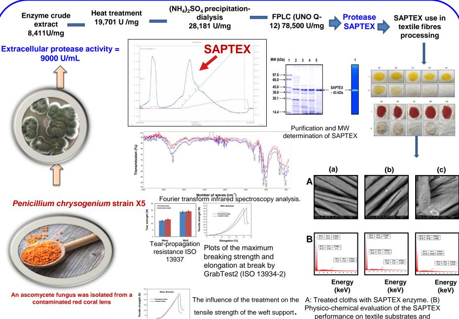
Physico-chemical evaluation of the SAPTEX performance on textile substrates and spectrophotometry analysis with dispersive energy.
