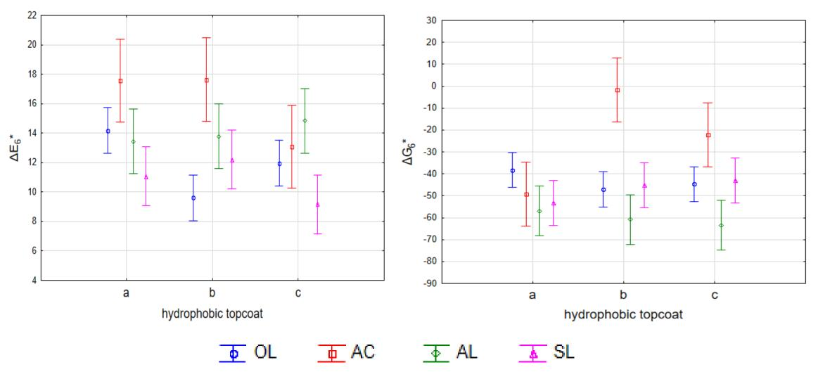
Efficiency of hydrophobic layer on the color and gloss change after 6 weeks of AW
