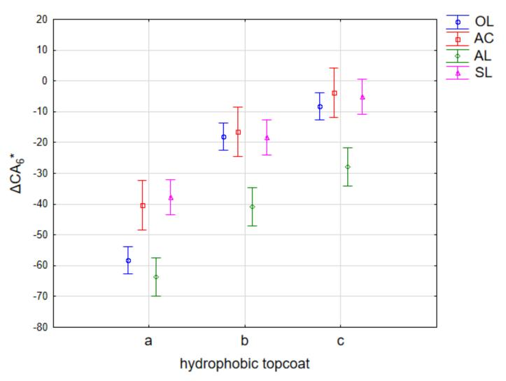
Efficiency of hydrophobic layer on the contact angle change after 6 weeks of AW
