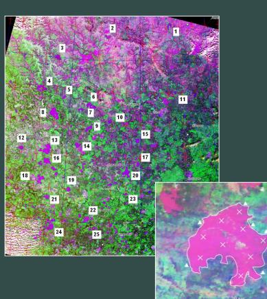
Test post-pyrogenic sites on the multispectral image of Terra / MODIS; Selection of points for measurement of temperature/NDVI. The averaged temperature and NDVI dynamics were investigated in total for 50 post-fire plots under different stages of succession (1, 2, 5 and 10 years after burning) in comparison with nondisturbed vegetation cover sites under the same conditions.
