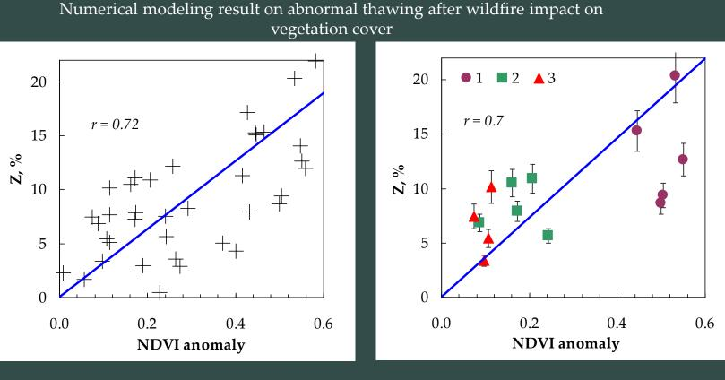
Increment of the thawing layer depth *vs* NDVI anomaly. Correlation of r=0.72
