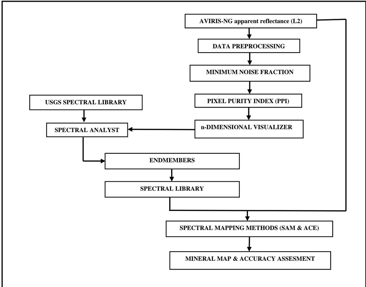
Figure 1. Flow diagram showing the methodology/algorithm adopted (Courtesy: ENVI 4.7 User's guide 2009).
