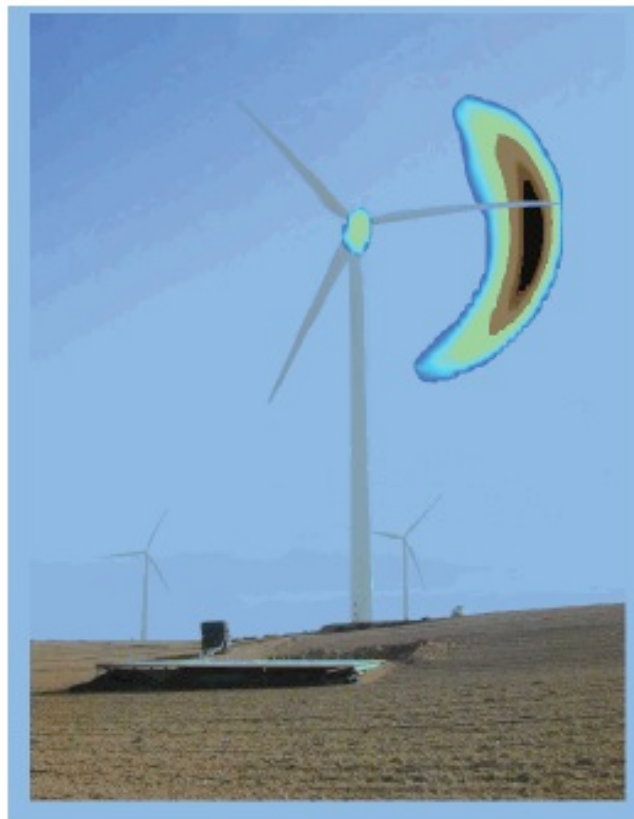
Figure 8. Area on a turbine blade with largest sound production [2].
