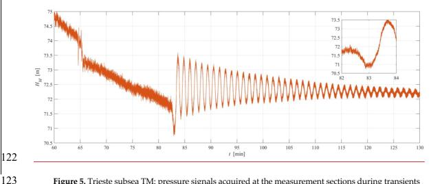
Figure 5. Trieste subsea TM: pressure signals acquired at the measurement sections during transients generated by the closure of the VM valve at "Molo 0". In the upper box a magnification of the first characteristic period of the pressure signal after the total closure of the valve VM is reported.
