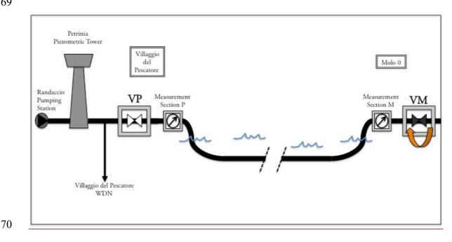
Figure 1. Schematic of the Trieste subsea transmission main (TM) managed by AcegasApsAmga SpA 72 (Hera Group).
