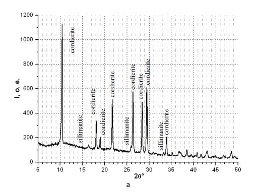
Fig. 12 Diffractograms of ceramics sample (a) and ceramic fibers (b)
