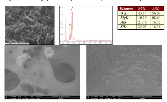
Fig. 11 SEM micrographs and X-ray elemental analysis of ceramics sample at 1300 °C
