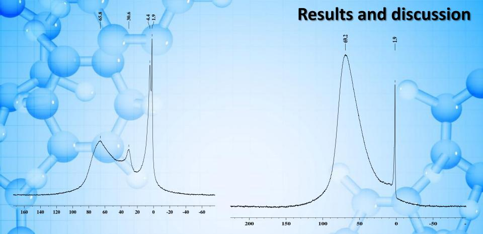
In <sup>27</sup>Al NMR spectra (600.13 MHz, CDCl<sub>3</sub>)of the concentrated oligomer solutions in CDCl<sub>3</sub> three types of signals of almost the same intensity are recorded: 70.0–80.0 ppm (4-coordinated), 30.0–45.0 (5- coordinated), 1.8-7.5 ppm (6- coordinated).
