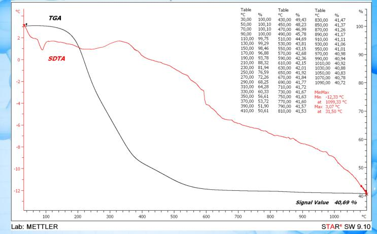
The TGA curve shows that the oligomer is stable when heated to a temperature of  $\approx 200 \ ^\circ$ C. The main weight loss occurs in the temperature range of 200–500  $^\circ$ C (the remainder is about 45 weight %). Further, the removal of residual hydroxyl groups in the form of H<sub>2</sub>O vapor is observed, the ceramic residue is 40.69 wt %, which corresponds to the theoretical values (slide 6).
