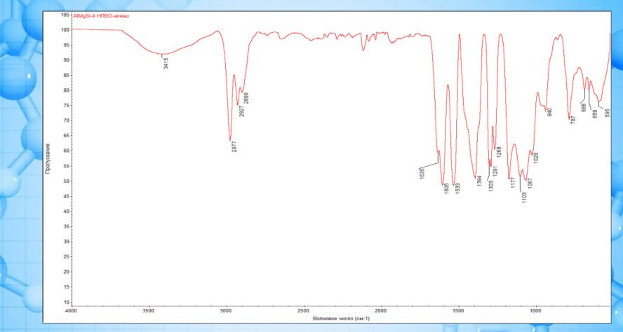
IR (cm<sup>-1</sup>): 595 v(Mg–O–Al), 659, 688 v(Mg–O; Al–O; Si–O), 863 v(Al–O–Al), 940 v(Mg–O), 967 v(Al–O<sub>4</sub>; Si–O), 1030, 1071, 1101, 1176 v(Mg–O–C; Al–O–C; Si–O–C), 787, 1268, 1291, 1303, 1398  $\delta$ {CH, C(CH<sub>3</sub>)} and v(C–O), 1533 v(C=C), 1602 v(C=O from [CH<sub>3</sub>(O)CCH=C(CH<sub>3</sub>)O]), 1635 v(C=O, bonded by coordination bond with Al atom), 2899, 2927, 2977 v(CH), 3415 v(OH)
