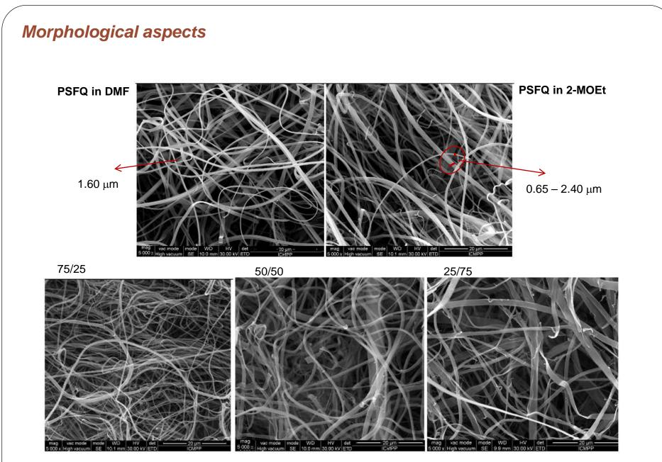
SEM images of PSFQ fibers obtained in: DMF and 2-MOEt at 40 g/dL polymer concentration for  $50 \mu m$  scan area and magnification of 2000x
