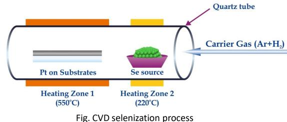
The CVD process is mediated via a carrier/reactive gas mixture flow of 95% Ar / 5%  $H_2$  for 2h with consequent formation of another necessary gaseous precursor -  $H_2$ Se to enable the PtSe<sub>2</sub> growth.
