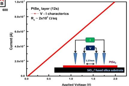
• Sheet resistance by four probe method V-A characteristics (Ohm contacts) and  $R_{s}^{\,\sim}\,2x10^{3}~\Omega/sq$
