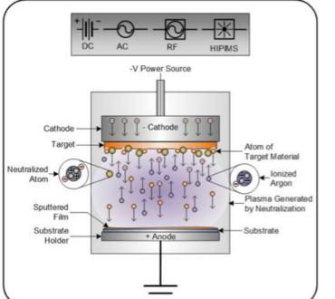
Fig. Magnetron spattering (charier-gas reactive conversion) www.semicore.com
