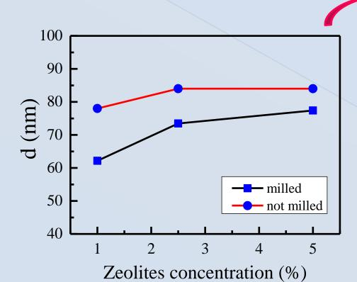
Dependence of thickness *d* on zeolite concentration (**b**) of thin  $Nb_2O_5$  films embedded with not-milled and milled fly ash FAU zeolites.
