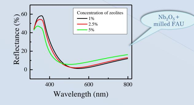
Reflectance spectra of  $Nb_2O_5\, films$  with milled zeolites
