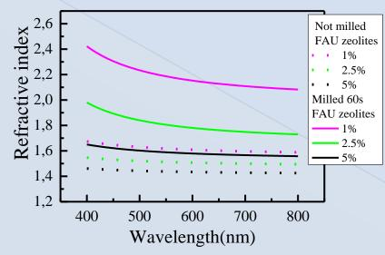
Dispersion curves of refractive index of thin  $Nb_2O_5$  films embedded with not-milled and milled fly ash FAU zeolites.
