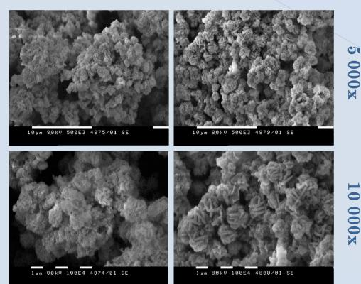
Agglomerations of indistinguishable particles are observed before milling and octahedral shape crystallites typical of the FAU phase.
