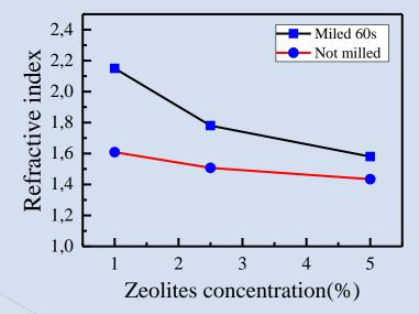
Dependence of refractive index n at wavelength of 600 nm on zeolite concentration of thin Nb<sub>2</sub>O<sub>5</sub> films embedded with not-milled and milled fly ash FAU zeolites.
