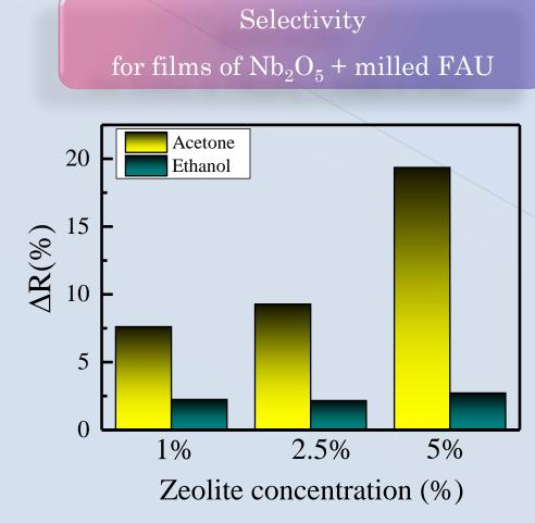
Zeolite concentration dependence of reflectance change induced by exposure to liquid acetone (yellow) and ethanol (green) of milled zeolites embedded in thin  $Nb_2O_5$  films. Measurements are conducted at room temperature.
