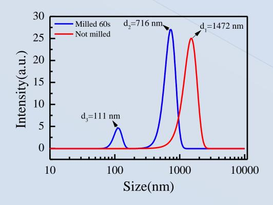
Size distribution changes from monomodal  $(d_1)$  in the case of non-milled zeolites to bimodal  $(d_2$  and  $d_3)$  for milled samples:
