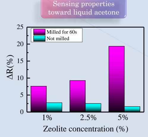
Zeolite concentration dependence of reflectance change induced by exposure to liquid acetone of FAU not-milled (blue bars) and milled (magenta bars) embedded in thin  $Nb_2O_5$  films. Measurements are conducted at room temperature.
