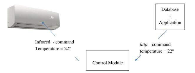
The database also stores the status of the drive modules to know in real time the situation of each device, when a controller module of the air conditioning is turned on, it announces itself to the system, recording date and time of activation.
