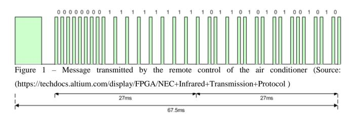
For this reason, a database was chosen, which stores the messages of the commands of each air conditioner. Thus, the microcontroller is responsible only for receiving the message via *http* protocol (hypertext transfer protocol) and sends it via infrared, simplifying complexity and reducing cost, and allowing easy scalability of the project.
