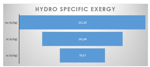
Figure 7. Hydraulic specific exergy, potential and thermal contributions.
