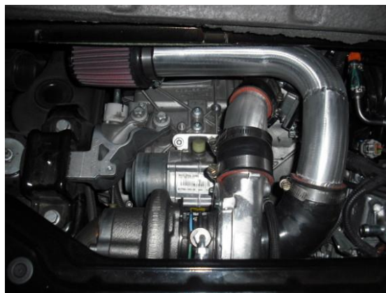
Figure 5. The turbocharged W451, 998 cc, 62 kW engine.
