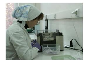
3. Assembling of a multimembrane composite and cutting it to individual test strips
