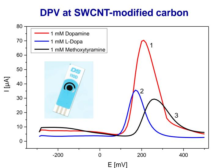
→ Current signal of L-Dopa and methoxytyramine in the potential range of the peak current of dopamine
