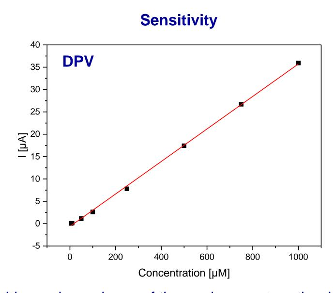
→ Linear dependency of the peak current on the dopamine concentration in the range from 5 µM to 1 mM
