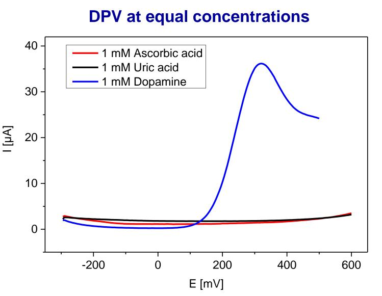
→ No oxidation current of ascorbic acid and uric acid in the potential range of the peak current of dopamine
