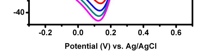
The voltammograms of bare gold electrode recorded in 5 mM (1:1)  $[Fe(CN)_6]^{3-/4-}$  as a redox probe in 0.05 M KCI solution at various scan rates.
