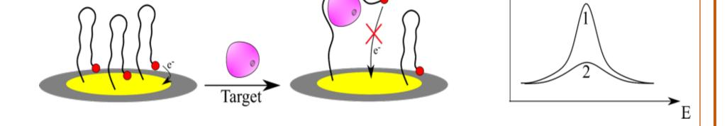
The scheme of electrochemical aptasensor. **Signal off:** binding reduces the current from the redox tag (red circle). Aptasensor before binding of target (part 1) and after binding the cells (purple object, part 2). DPV current changes correspond to binding phenomenon.
